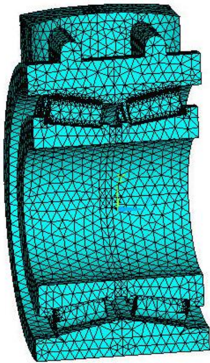
Fig. 6.15. Finite element model of a bearing assembly with a double-row conical bearing
