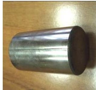
Fig. 2.9. Cracks and breaks in bearing rings and rollers
