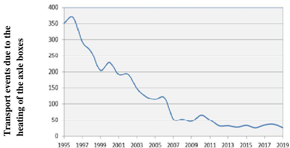
Fig. 2.5 Dependence of the change in the number of uncoupling of wagons on the route due to the heating of the axle assemblies
