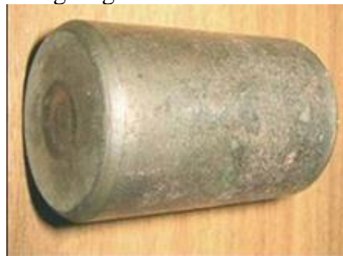
Fig. 2.10. Corrosion shells and pitting on bearing rings and rollers
