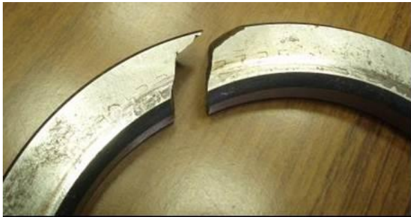
Fig. 2.9. Cracks and breaks in bearing rings and rollers
